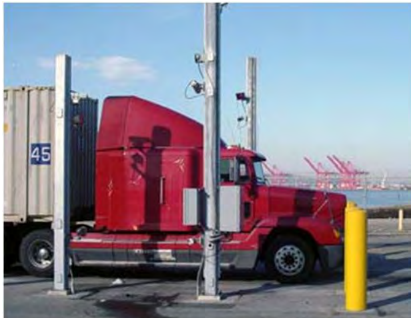
Figure 10-1: OCR technology automatically identifies equipment at the gates and on the quay
