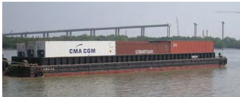
Figure 2-26: Example of a Non Self-Propelled Container Barge Operating in HCMC Region
