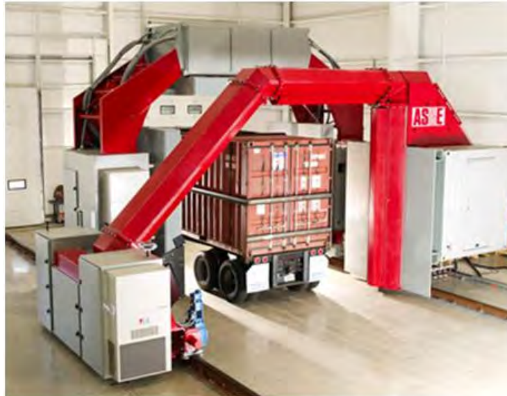
Figure 10-3: Stationary Vehicle and Rail-Mounted Inspection Portal
